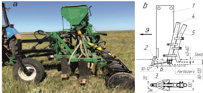
Figure 1 (a) The experimental model of the sod seeder. (b) The design scheme of the experimental hoe opener: 1 – shank; 2 – point; 3 – knife; 4 – fertilizers tube; 5 – seeds tube; 6 – spreader
